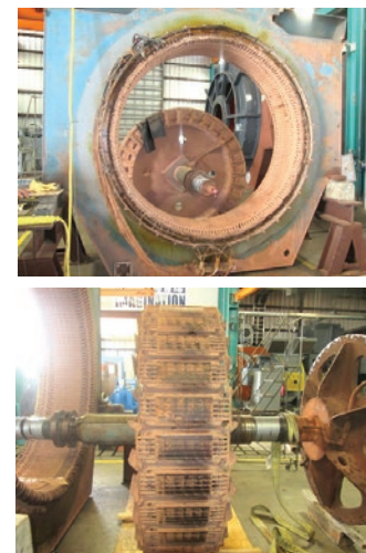
Figure 2: ALCOA windings covered in particulate
