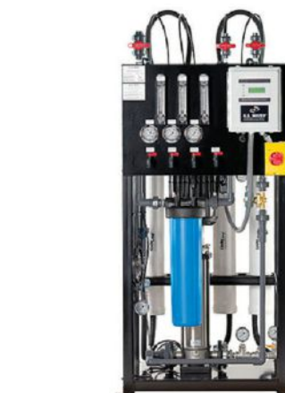
Figure 1: Example of a pilot RO system. The pilot RO system should duplicate the permeate recovery, the permeate flux rate (that is, the permeate flow per unit of membrane area), and concentrate stream vessel exit velocities, along with the scale inhibitor dosage and shutdown flush methods.
