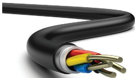
Silane crosslinking is an established process that improves the performance of cables. In comparison to thermoplastic polymers, crosslinked polymers achieve much better results when it comes to resisting heat, deformation, and weather effects.
