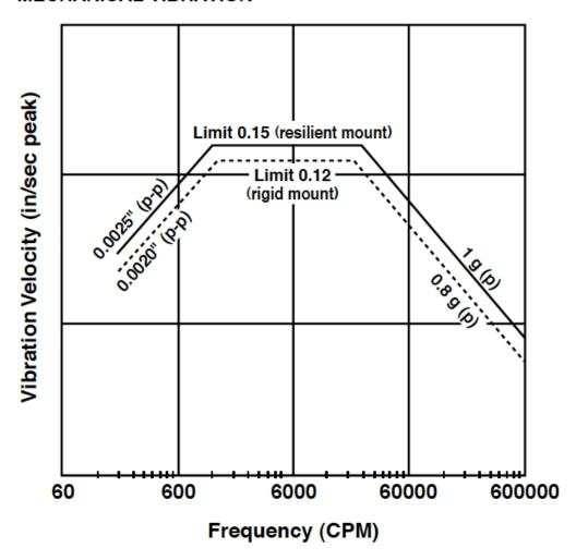
Note: The intersection of constant displacement lines with constant velocity lines occurs at approximately 1200 CPM. The intersection of constant velocity lines with constant acceleration lines occurs at approximately 24000 CPM.
